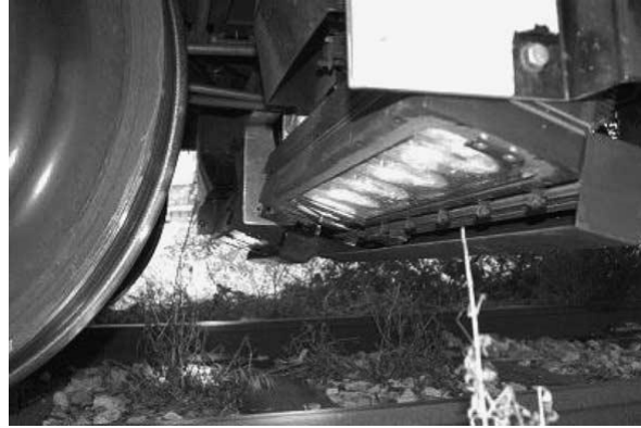
(b) An image acquisition system installed under a rail inspection car for automatic visual inspection
