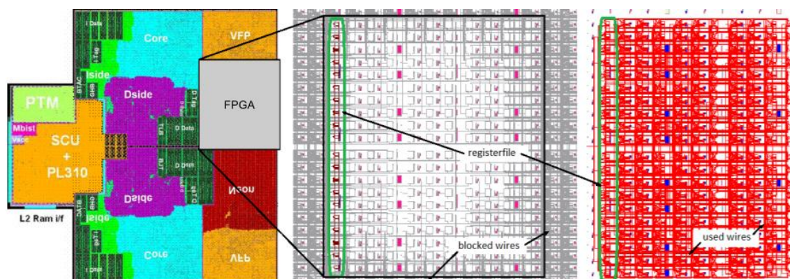
Figure 2.1: ARM Cortex A-9 Macrocell Floorplan edited to highlight FPGA Interlay concept on a SoC [10].
